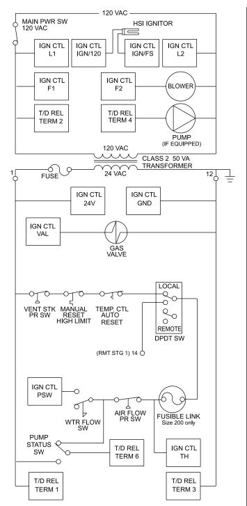
Figure 17. Logic Diagram, ON/OFF Boiler or Water Heater.
